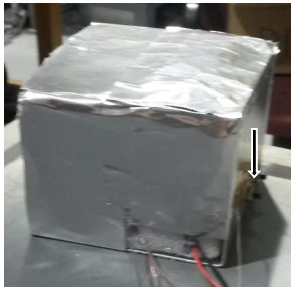
Figure 7. Overall test bed assembly. Thermocouple mounting location indicated by arrow. Note Styrofoam insulation (mostly covered by aluminum tape but visible in bottom-right corner).
