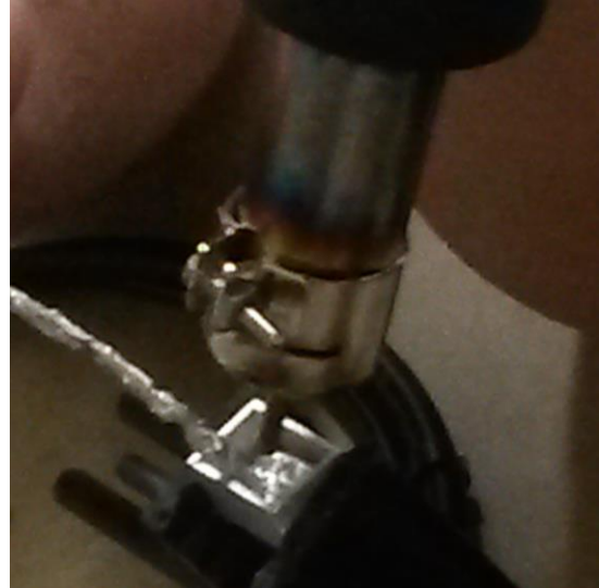
Figure 4. Manual melting of solder (PCM) ribbon into heatsink using a heat gun.
