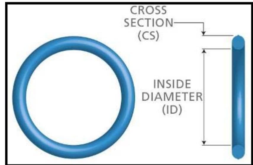
Figure 1: True O-Ring Profile<sup>1</sup>
