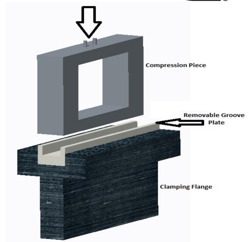
Figure 6: Test Fixture Prototype
