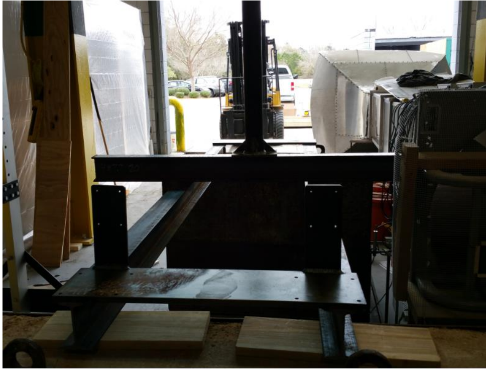
Figure 13 Gantry load testing (Experiencing 2500 lbf load)
