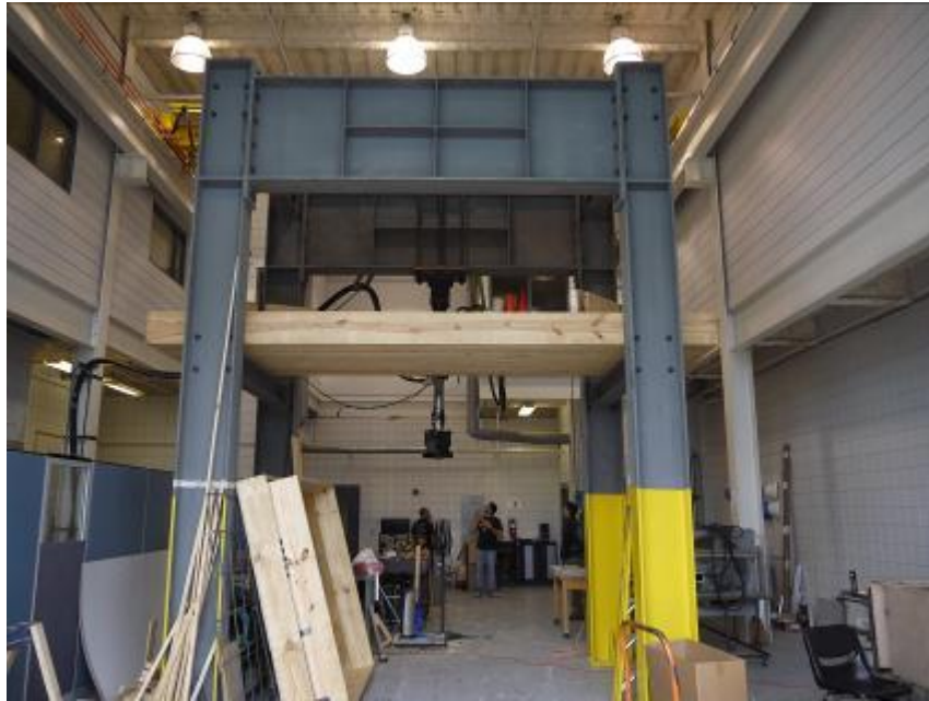
Figure 12 MTS actuator in the civil engineering Structures Lab
