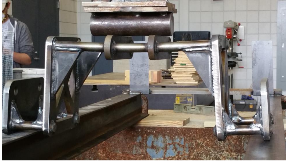
Figure 14 Magnified View of trolley load testing (Experiencing 2500 lbf load)
