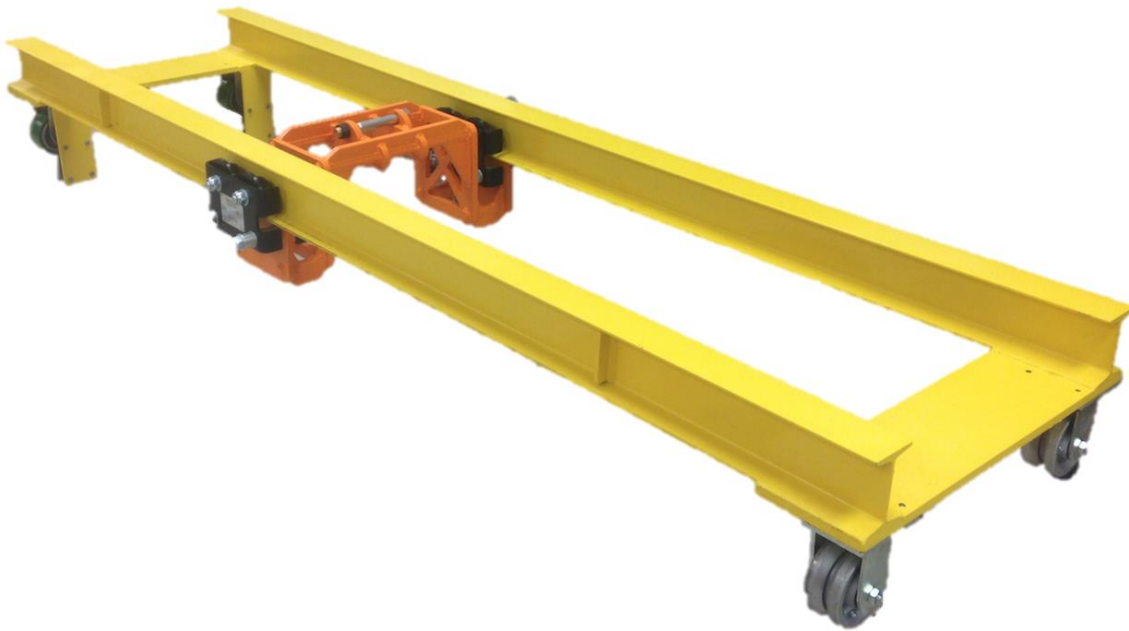
Figure 7 Picture of the painted and fully assembly gantry and trolley system
