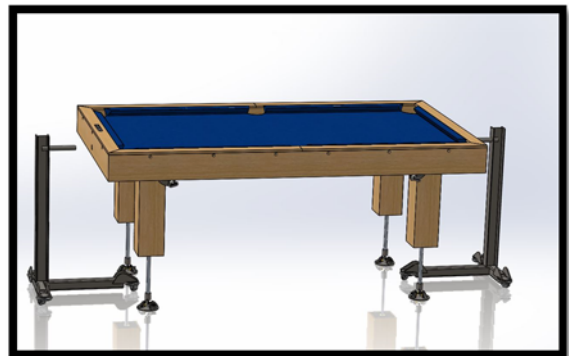
Figure 4: The two dollies rolled up to the pool table in order to attach and
