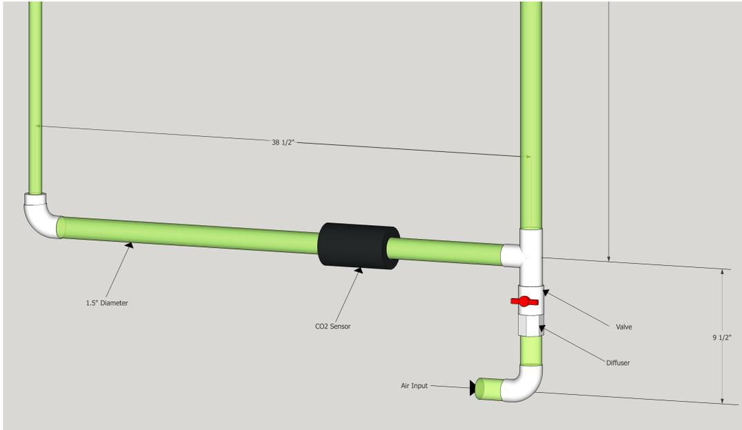
**Fig 4A:** Top half of photobioreactor.
