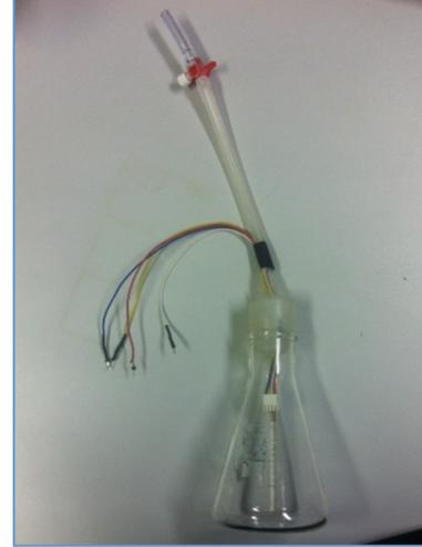
Fig 6: Airtight beaker with sensor.
