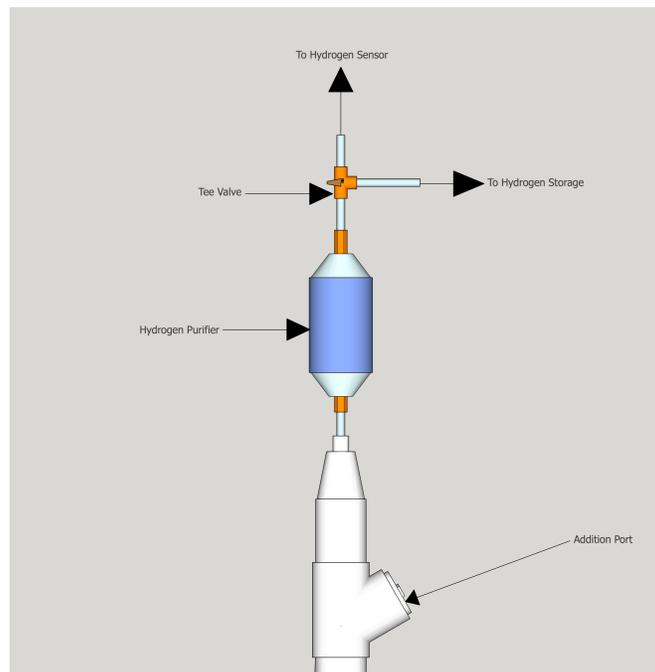
**Fig 2A:** Components and connection of degassing column.
