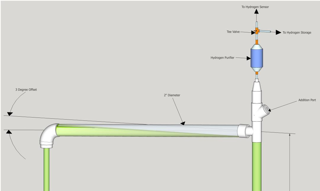
**Fig 3A:** Top half of photobioreactor.
