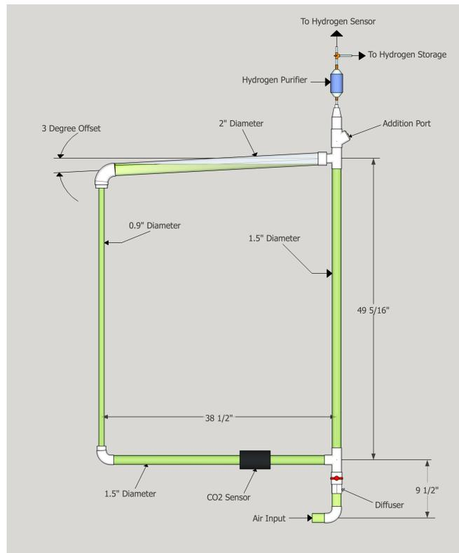
**Fig 1A:** Front view of photobioreactor with dimension
