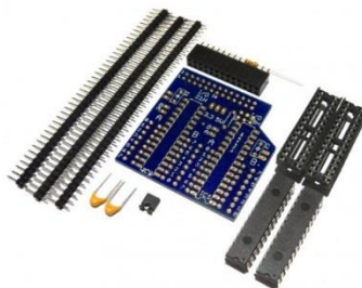
Figure 1 - MyPi - Protect Your Pi - 32 I/O Point Expansion & GPIO Shield Board
