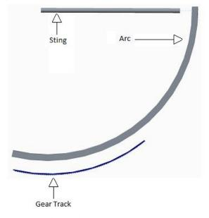
Figure 2: Arc-sting assembly
