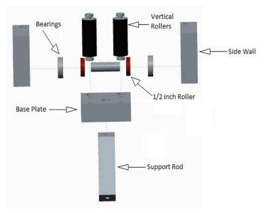
plate. It is imperative that the support Figure 5: Follower Assembly
