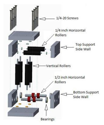
Figure 3: Housing assembly
