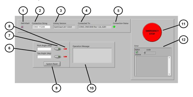
Figure 7: LabVIEW User Interface (Front Panel)
