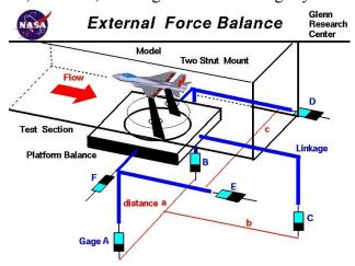
**Figure 2: External Force Balance<sup>4</sup>**
