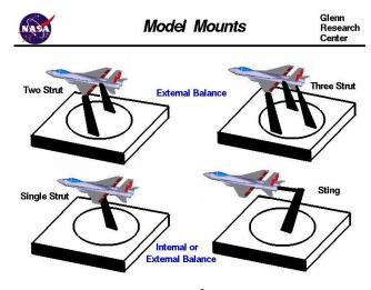
Figure 1: Model Mounts<sup>2</sup>
