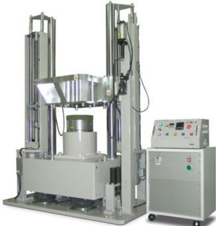
Figure 1: SDST: Single drop shock test apparatus [6]
