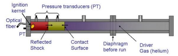
Figure 1 - Example of a Shock Tube [10]
