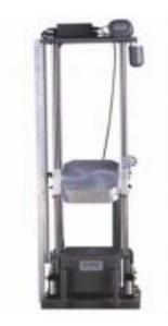
Figure 2 - Example of a Drop Table [12]
