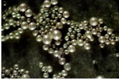
Figure 1. Optical microscope image of SLMP taken from FMC
