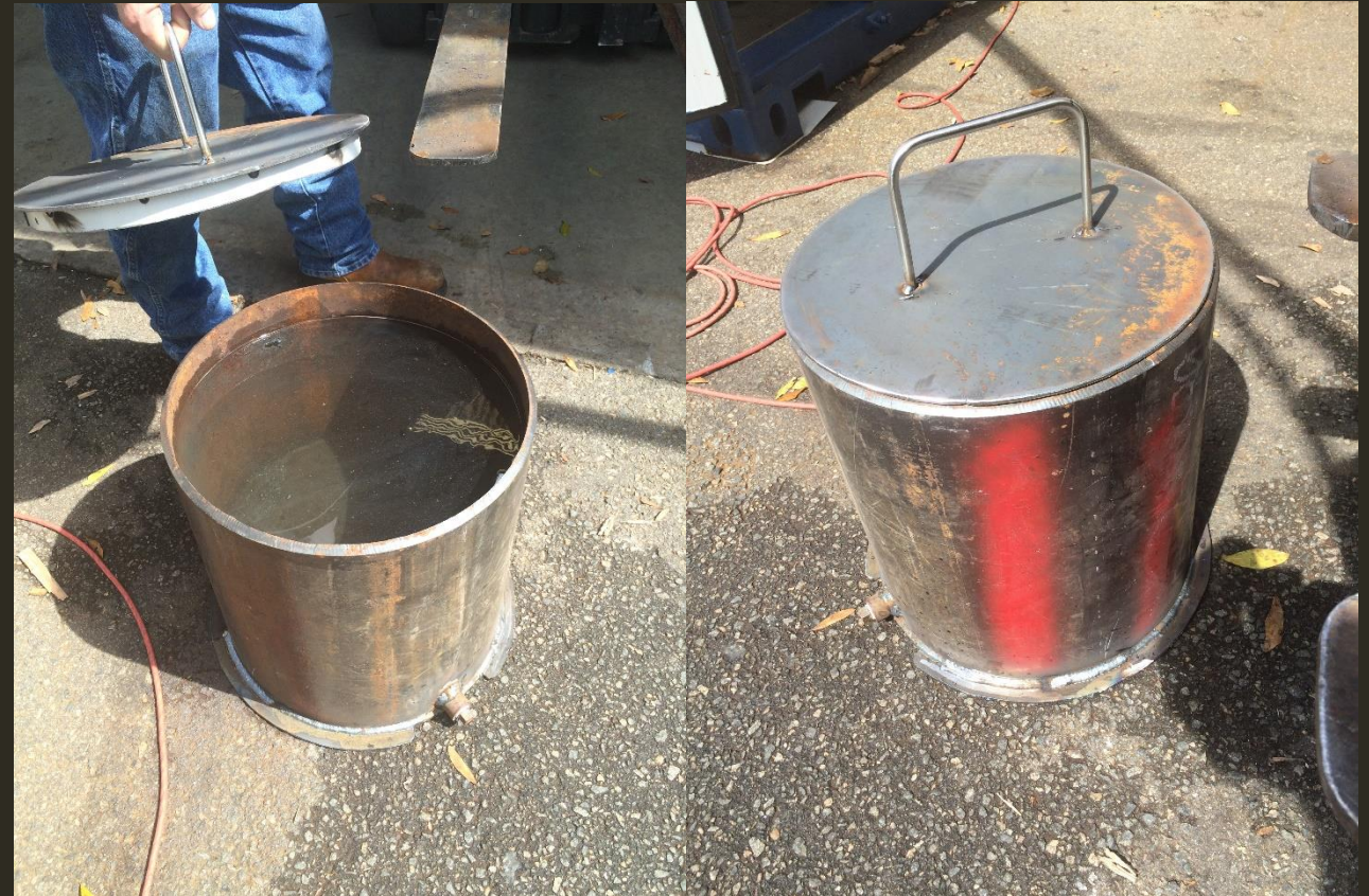
Figure 16. Final tank assembly
