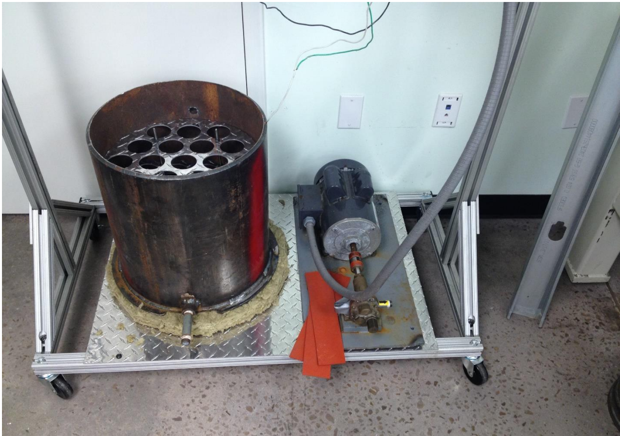
Figure 1. Tank with Baffles frame installed
