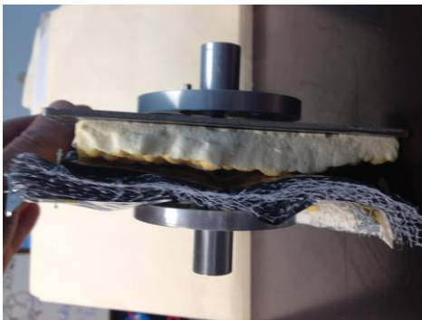
Figure 2: Layers of insulation currently in place surrounding a cryogenic tank
