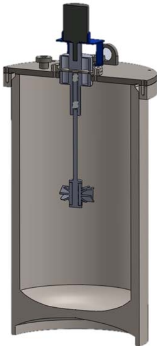
Figure 11: Design proposed by the group utilizing an axial pump.
