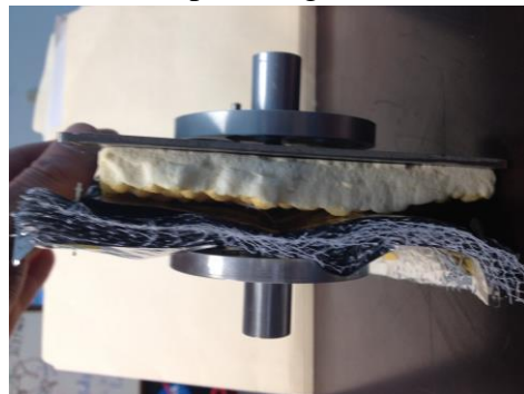
Figure 2: Layers of insulation currently in place on cryogenic tank
