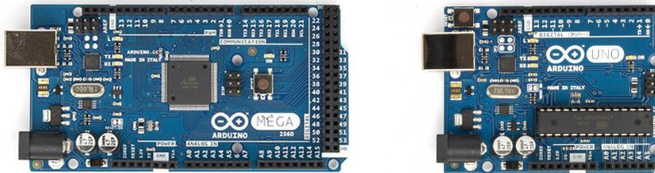
Fig. 3.2.2: (Left) Arduino Mega 2560 Rev3; (Right) Arduino UNO Rev3
