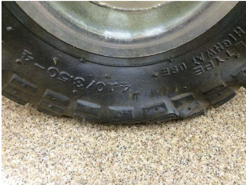
Figure 9. Zoomed in view of the deflated wheels from the previous year's mechanism
