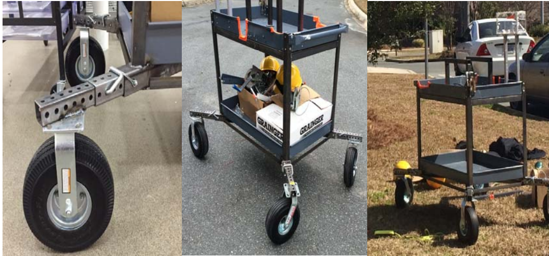
Figure 18. The wheels being tested on different terrain (concrete, asphalt, and grass/dirt)
