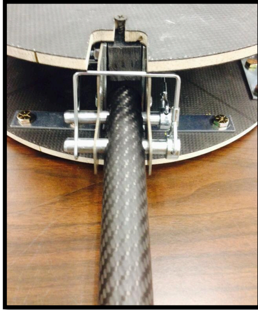
Figure 61. Lock Arm into Horizontal Position
