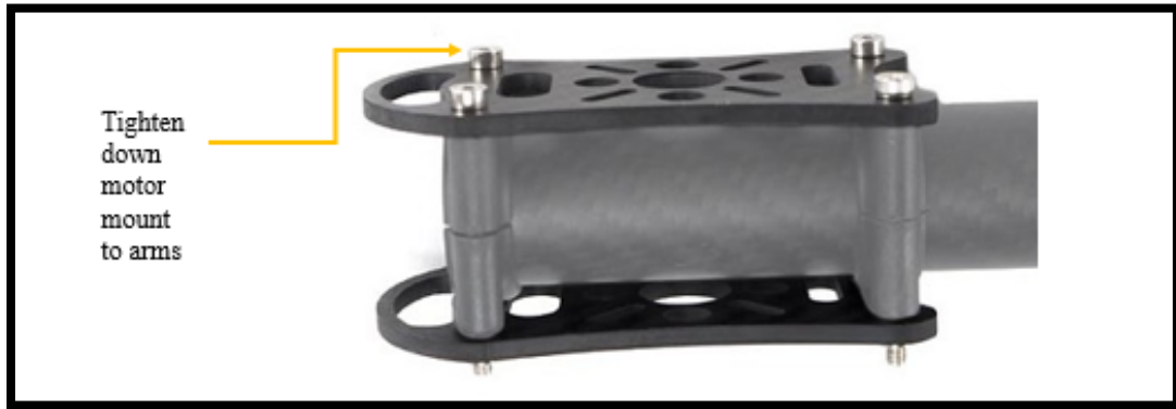
Figure 53. Secure Motor Mount to Carbon Fiber Arm
