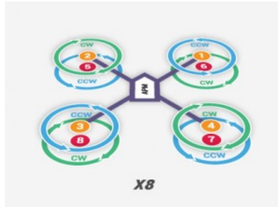
Figure 9. Coaxial Configuration of Eight Motors on Four Booms
