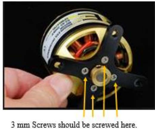
Figure 23. Mounting Prop Mount to Motor
