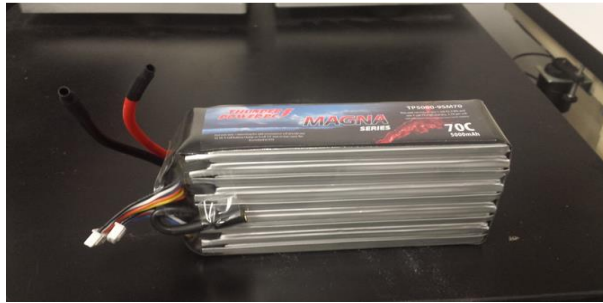
Figure 20. Thunder Power 33.3 V 9S Lithium Polymer Battery
