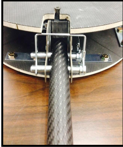
Figure 61. Lock Arm into Horizontal Position
