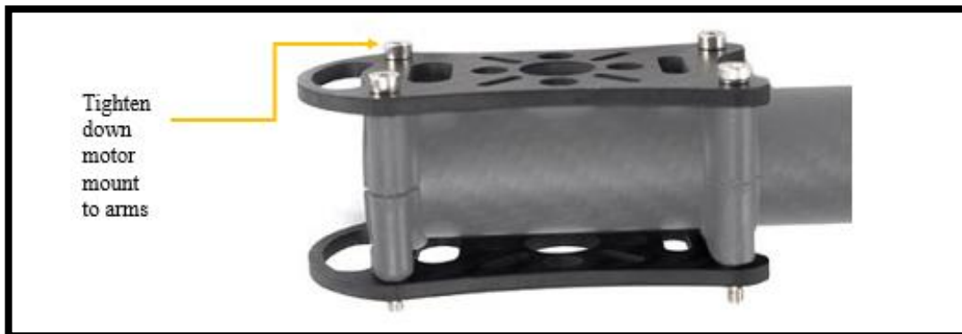
Figure 53. Secure Motor Mount to Carbon Fiber Arm
