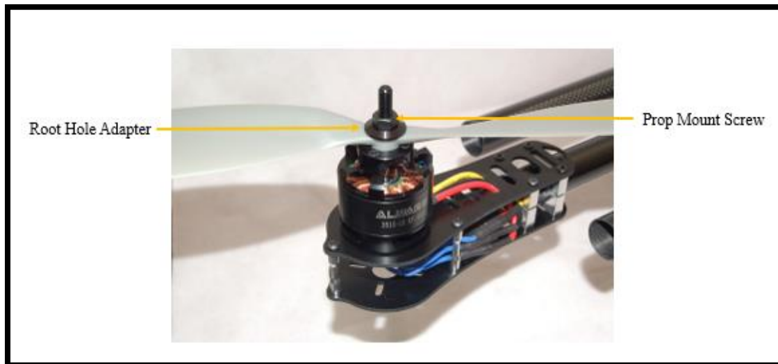
Figure 55. Install Propeller on Motor
