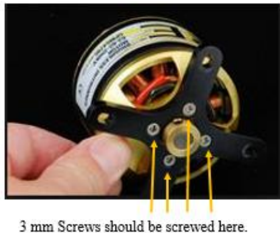
Figure 48. Mount Propeller Mount to Motor
