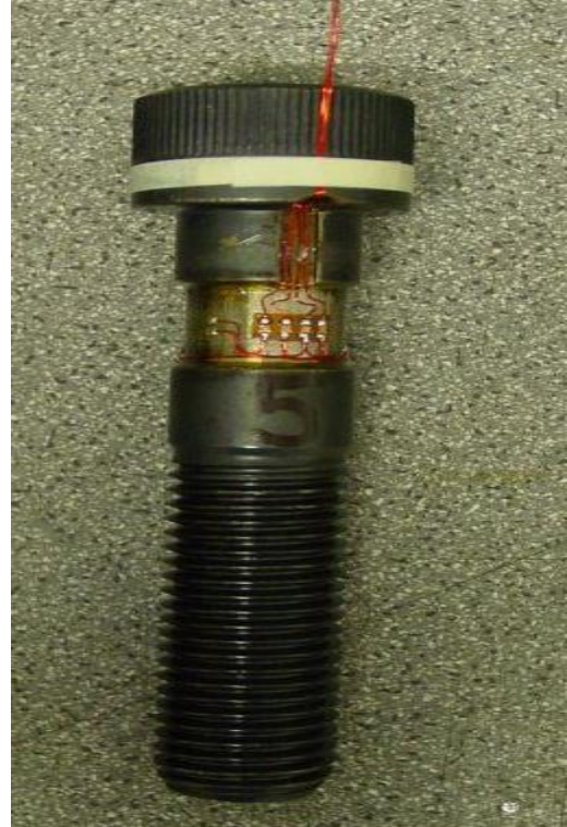
Figure 2. Modified bolt with strain gauge.
