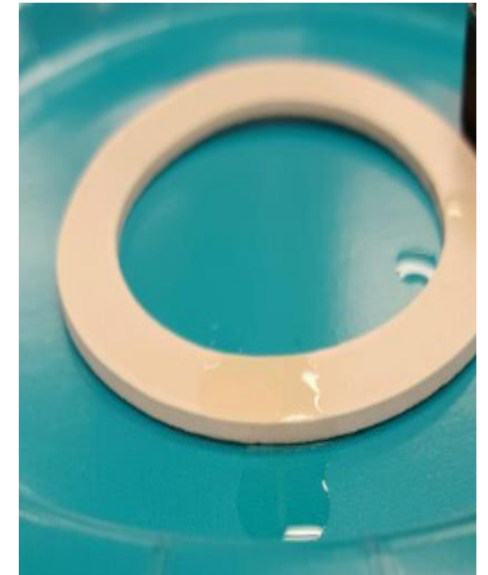
Figure 24. Teflon gasket after oil removal
