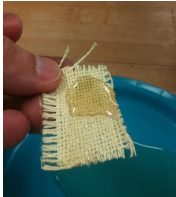
Figure 22. Fiber cloth material after impregnation and oil droplet dispersed
