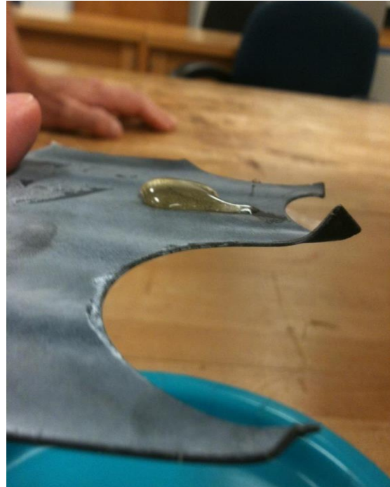
Figure 15. RCM gasket after spray and oil droplet dispersed
