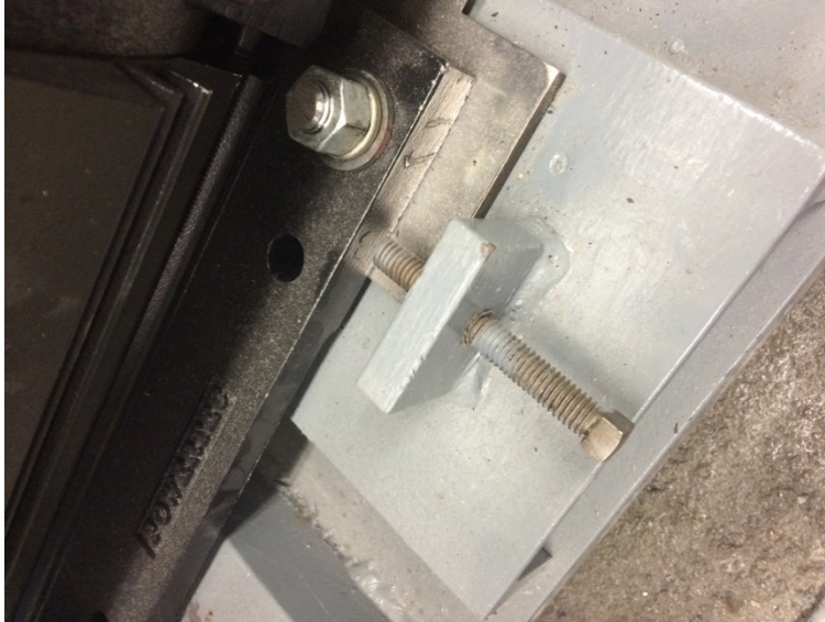
Figure 6. Lateral adjustment with set screws and motor mounting bolt.
