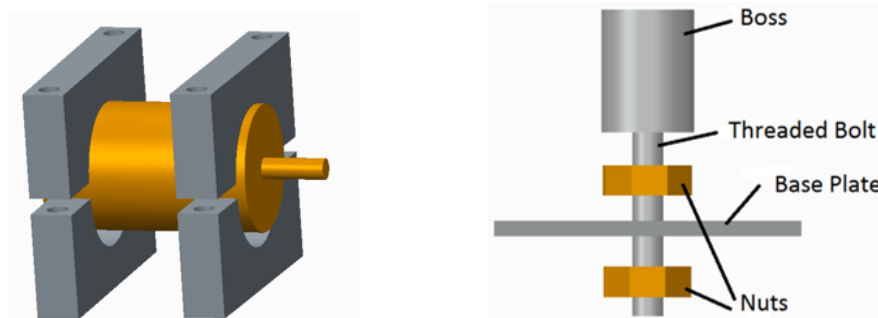
Figure 10. Left: DC Motor Camps. Right: Elevation adjust system.
