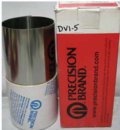
Figure 17, 18 & 19. Shim stock(left), shim dimensioning (center), shim location (right).
