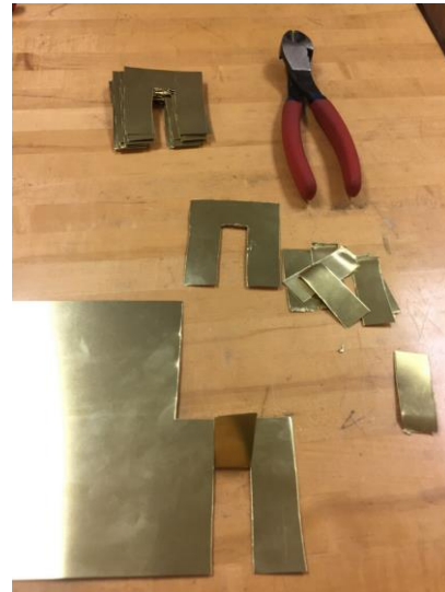
Figure 17, 18 & 19. Shim stock(left), cut shims (middle), shim location (right).
