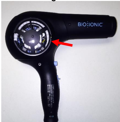
Cover and baffle removed from intake
