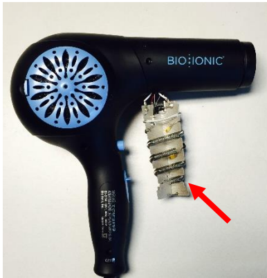
Heating element removed for unimpeded flow through nozzle
