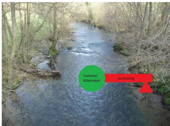
Figure 14 - Cantilever style anchoring
