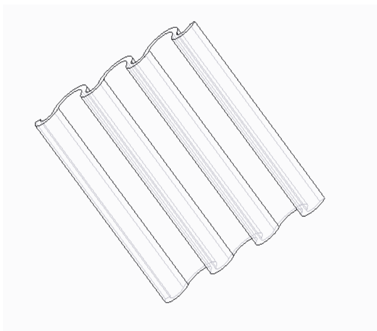
Fig c5. Concept cad of corrugated lamellae structure.
