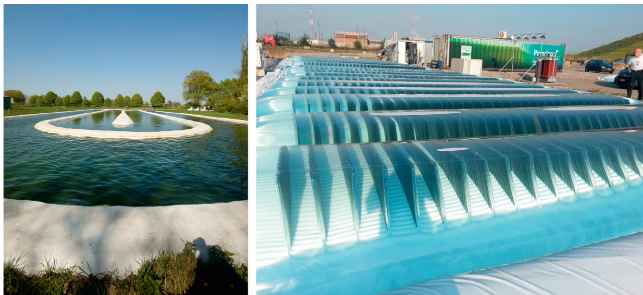
Figure 1. Example of open 'raceway pond' reactors (Ingrepo, The Netherlands) and a novel design of a low-cost photobioreactor (Proviron, Belgium).
