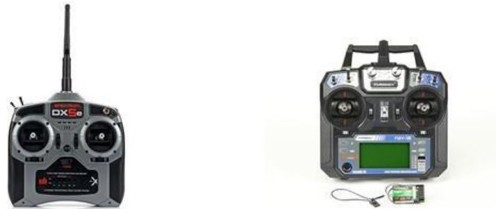
Figure 7: Spektrum R5520 DX5e DSMX Transmitter (left) and Turnigy TGY-i6 AFHDS Transmitter (right).
