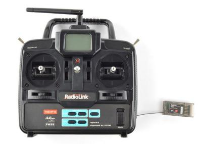
*Figure 9: Robo-Weeder Transmitter and Receiver.*
