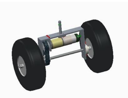
Figure 8: Robo-Weeder Drive Mechanism.
