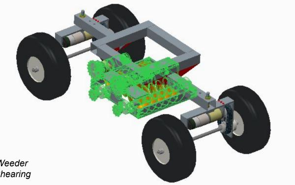
*Figure 3:* Robo-Weeder with Highlighted Shearing Mechanism.
