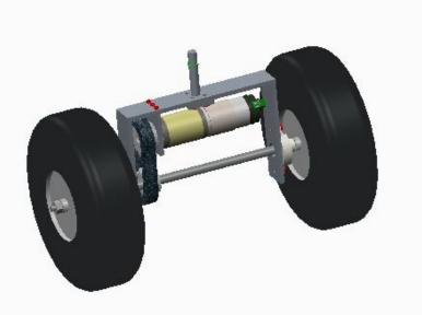
Figure 8: Robo-Weeder Drive Mechanism.
