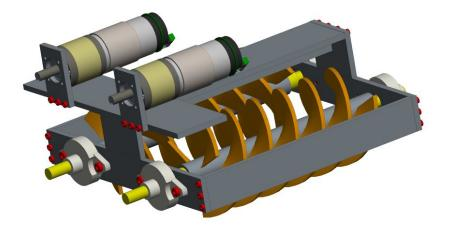
Figure 4: Fully Assembled Shearing Mechanism.
