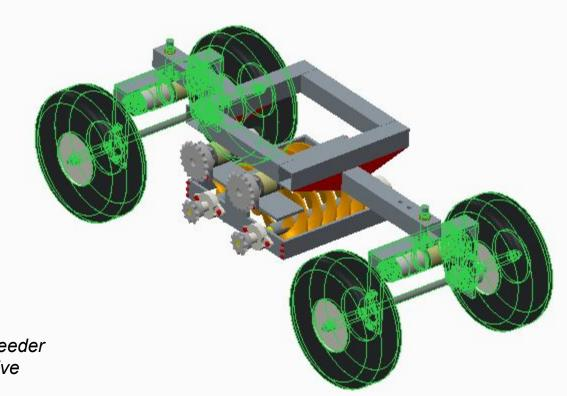
*Figure 7:* Robo-Weeder with Highlighted Drive Mechanism.
