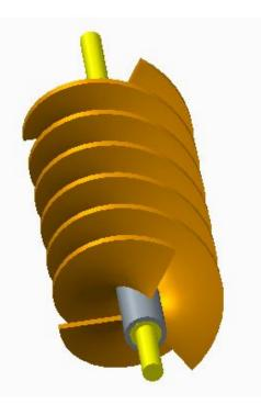
Figure 5: Custom Auger Assembly
