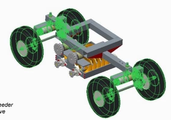
*Figure 7:* Robo-Weeder with Highlighted Drive Mechanism.
