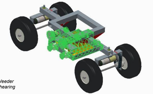
*Figure 9:* Robo-Weeder with Highlighted Shearing Mechanism.
