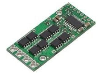
Figure 11: Motor Driver for use on the Robo-Weeder.
