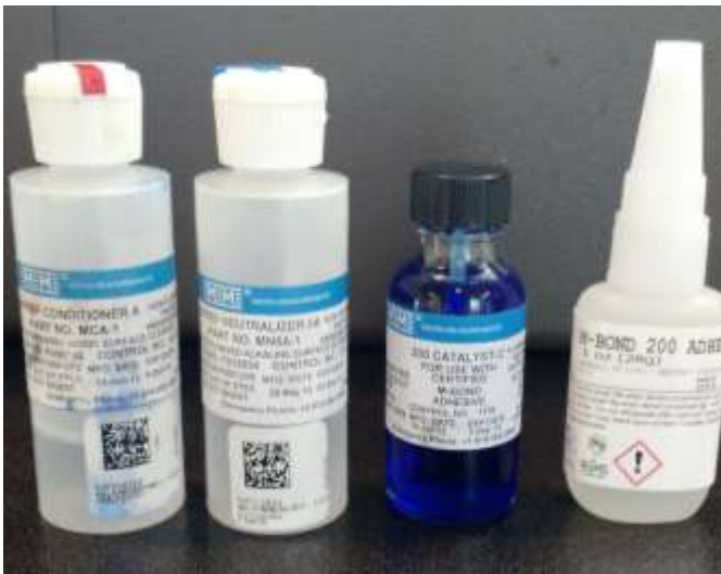
Figure 1. Strain Gauge Application Materials
