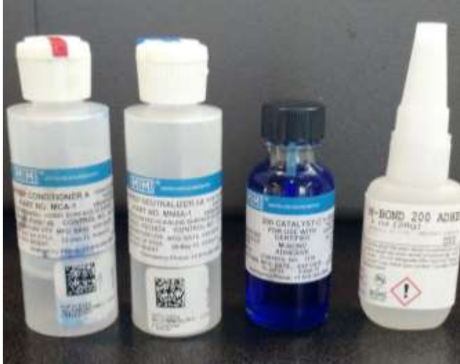
Figure 9. Strain Gauge Application Materials.
