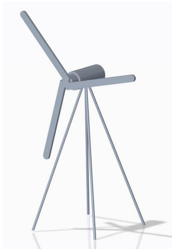
Figure 1. Bodiless wind turbine concept.
