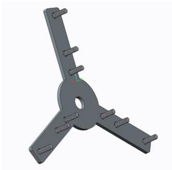
Figure 31. Final hub assembly that will be used to mount the blades to the Portable Wind Turbine Prototype.
