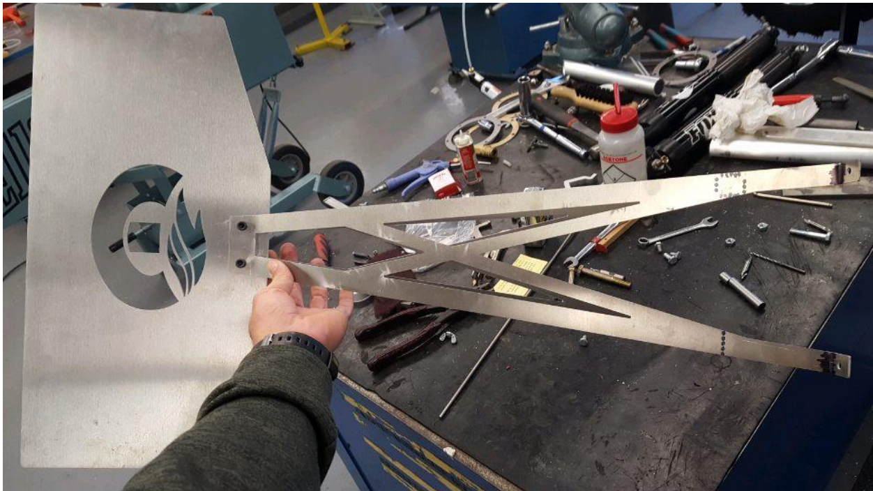
Figure 50. Tail vane assembly held by a team member in the FAMU-FSU College of Engineering Machine shop.
