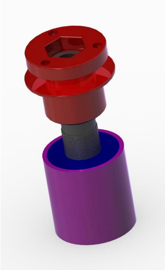
Figure 6. The quick release nacelle mounting system.
