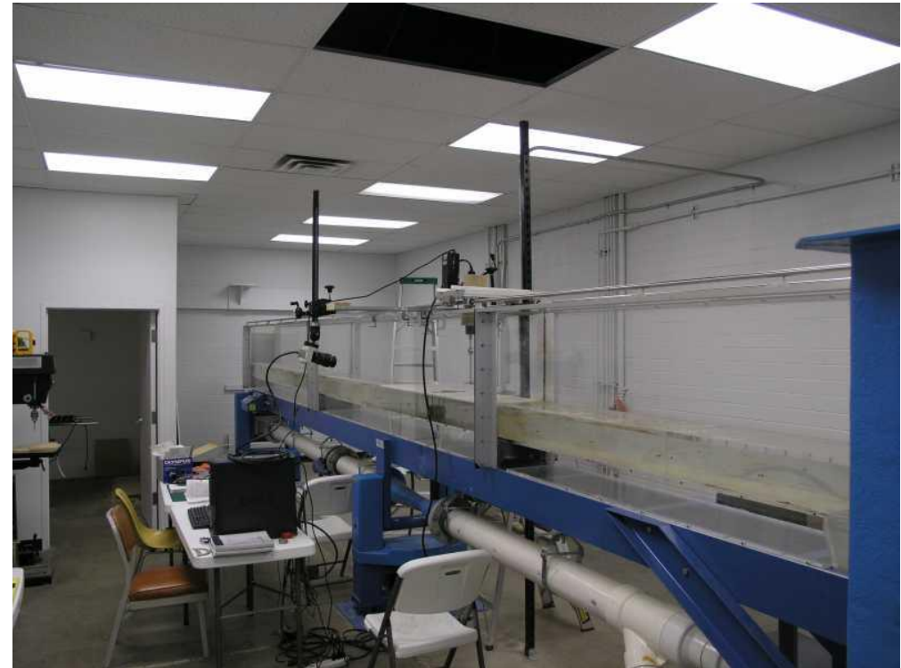
Figure 5: Flow Flume in physics building
