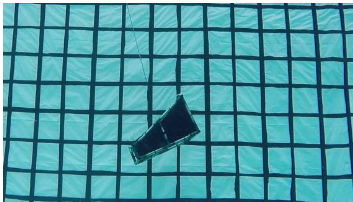
Figure 19: Snap shot of the video of the second round of testing. Shows trapezoidal model being pulled through pool. Back drop was used as reference to measure tilt. Drag surface was attached to the top during this test, resulted in a greater angle of tow.
