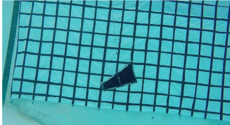
Figure 18: Snap shot of the video of the second round of testing. Shows trapezoidal model being pulled through pool. Back drop was used as reference to measure tilt. No drag surface was attached to the top during this test
