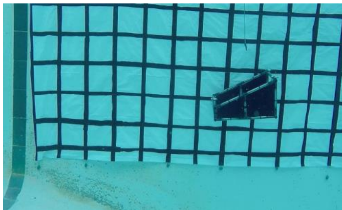
Figure 20: Snap shot of the video of the second round of testing. Shows trapezoidal model being pulled through pool. Back drop was used as reference to measure tilt. Drag surface was not attached to the top during this test, but the bridle cable lengths had been augmented, resulted in a very level tow.
