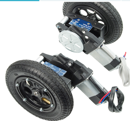
Example of differential steering
