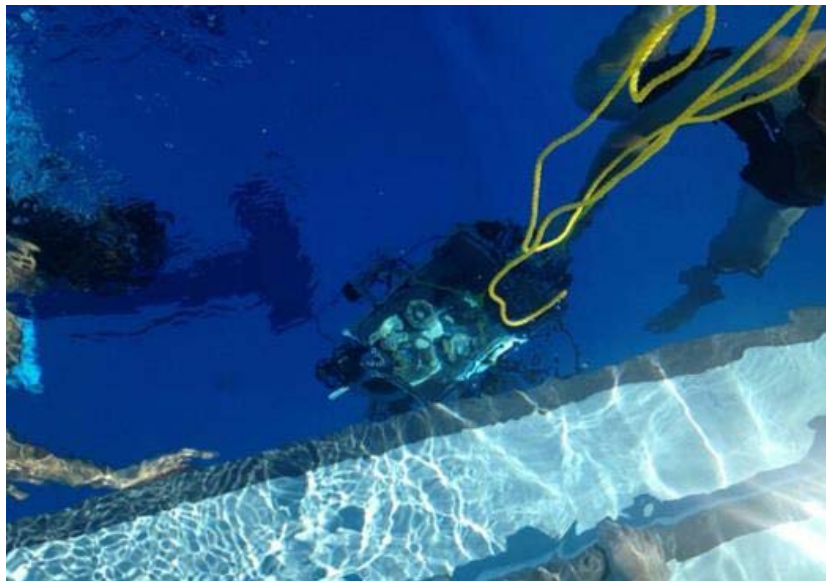
Figure 3: Buoyancy and leak testing at Morcom Aquatic Center 10/16/15
