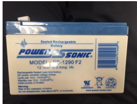
Figure 16: Power Sonic 12V battery
