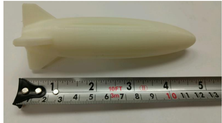
Figure 10: 3-D printed torpedo
