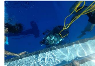
Buoyancy and Leak Testing at Morcom Pool
