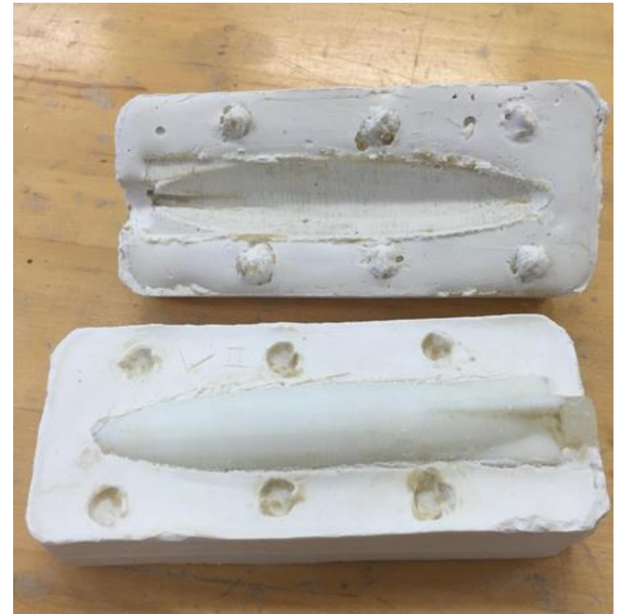
Figure 8: Torpedo Plaster Mold
