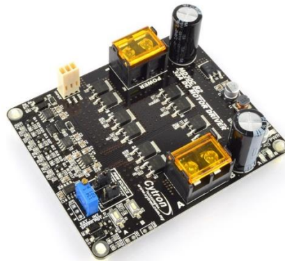
Figure 28: Motor Driver for Winch Motor [32]
