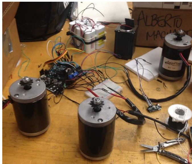
Figure 60: Functionality Test for Motor Drivers and Motors
