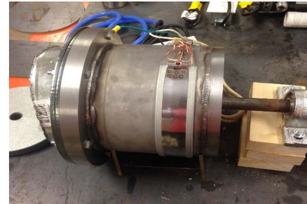
Figure 9: Picture of the custom crankcase employed in the test rig.
