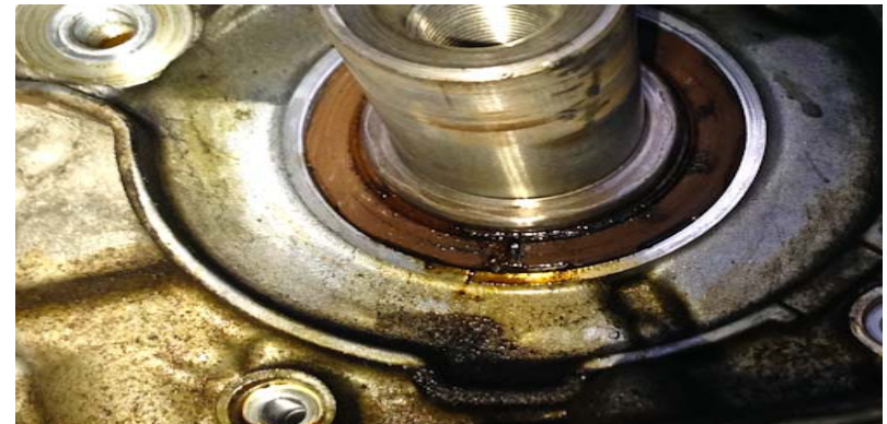
Figure 1: Depiction of rear crank seal leaking oil. 2
