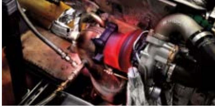
Figure 1: Depiction of a turbocharger during operation. The intense heat generated can be seen by the color change.
