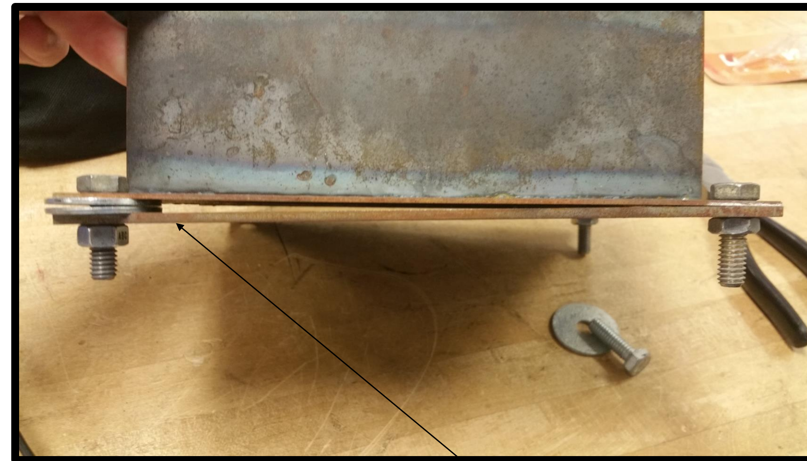
Not flush and parallel between engine block and intake manifold
